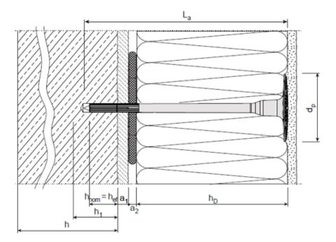
h<sub>nom</sub> = overall plastic anchor embedment depth in the base material
